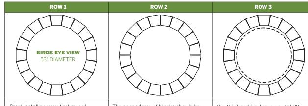
Start installing your first row of blocks by placing your first stone on the compacted base.
