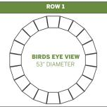
Start installing your first row of blocks by placing your first stone on the compacted base.
