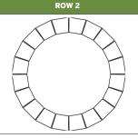
The second row of blocks should be staggered vertically from the row below.
